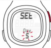
Press the START/STOP button. "Day" is displayed. Press the TOGGLE (-) or TOGGLE (+) button repeatedly to set the day.
