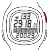
Press the START/STOP button. The running time begins. A stopwatch icon appears at the bottom of the display and the name of the measured value has a light background.
