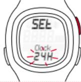
Press the START/STOP button. The time is displayed. The hours entry flashes.
