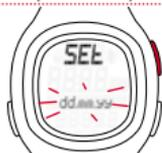
Press the START/STOP button. A date format is displayed. Select the desired date format by pressing the TOGGLE (-) or TOGGLE (+) button.
