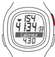
5. To finish training, simply press the START/STOP button. The stopwatch stops. To reset the values to zero, press and hold the START/STOP button. To exit the training mode, press and hold the TOGGLE (-) button.
