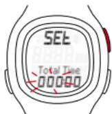
Press the START/STOP button. You will see zeros below the total time. The first three digits for the hours flash.
