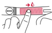
Lift the belt slightly from the skin and wet the rear surface of the conductive ribbed rubber pads with water or moisten the pads with saliva.
