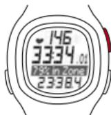
Hold down the TOGGLE [-] button. You switch to sleep mode. Only the time and date are displayed so as to save the battery. The current training values remain saved.
