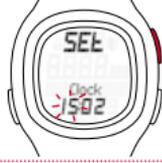
Press the TOGGLE (+) button. The hour increases by one. Press the TOGGLE (-) button to decrease the displayed hour by one.
