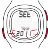
Press the START/STOP button. "Year" is displayed and below it the preset year flashes. Press the TOGGLE (-) or TOGGLE (+) button repeatedly to set the year.
